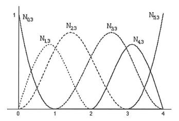
Using this figure, determine the following parameters of the curve: number of control points, order and degree of the curve, and the knot vector. Explain how these parameters are derived.
