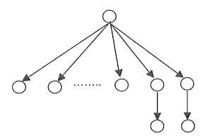
The graph consists of tasks that all have unit execution times. The nodes of the graph are mapped (by some scheduler) onto the parallel processor (we assume that every processor has at least one task assigned). The communication times between the processors can be neglected.
