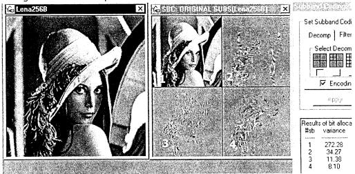
Each of the subbands will be PCM + Huffman encoded, such that the average bit rate is 1.5 bit per pixel
