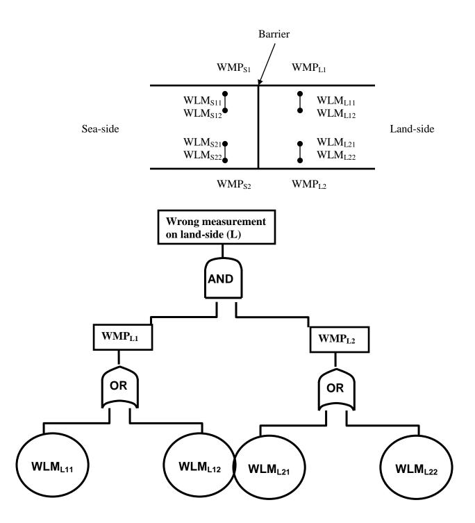
The part of FT for wrong measurement on the land side (L) is shown on the Figure above. Similar part of FT for the wrong measurement on the seas side (S) should be drawn. These two intermediate events should be connected by OR gate. Hence the probability of failure of the Storm Surge Barrier in the New Waterway near Rotterdam (FB) is:
