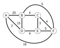
If we calculate the shortest path between A and F in this graph using Dijkstra's algorithm, how many times do we need to update the distance that is stored for node B (including the update from  $\infty$  to an initial value)?
