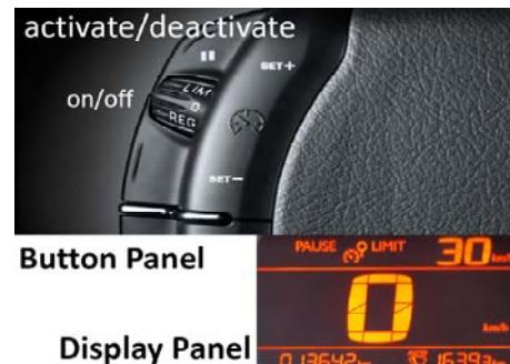
This figure illustrates the button panel and the control panel used for the SDS. “Reg” is intended for the speed regulator functionality (cruise control). The display shows the speed in the centre, and the data for the SDS at the top.
