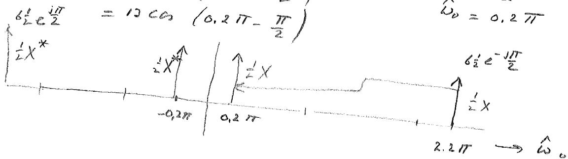
c)  $f_s = 15 \text{ Hz} \quad \text{undersampling (folding)}$
