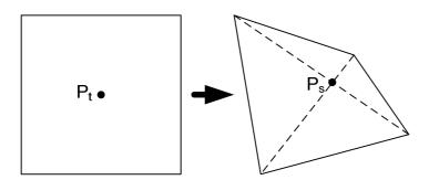
For which type of mapping the centre  $P_t = (0.5, 0.5)$  of the texture is mapped on the intersection P<sub>s</sub> of the diagonals of the quadrilateral in screen space?
