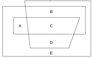
How many of the areas A, B, C, D and E in the figure above, showing a polygon with intersecting edges, are <u>inside</u> the polygon when using the *odd even* rule?
