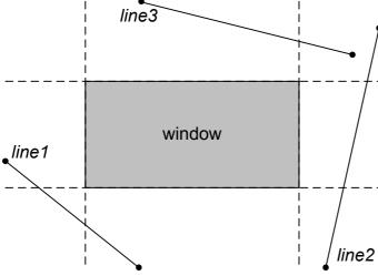
For how many of these lines no intersection points with horizontal or vertical window boundaries need to be calculated during the clipping process?
