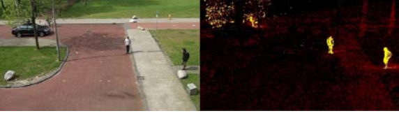
Figure 3: A camera image and the result of the MoG background subtraction. Yellow pixels represent detected foreground.
