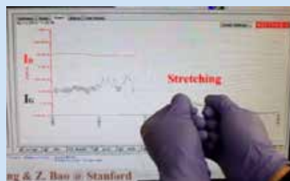
Figure 2: Researcher demonstrating the conductivity while stretching the polymer [5]
